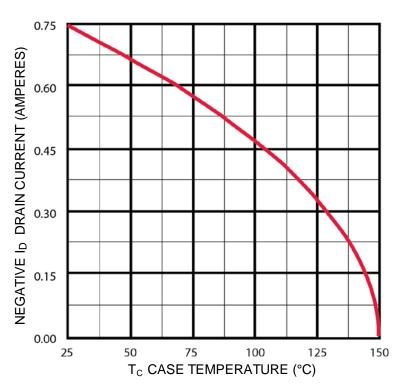
FIGURE 1 – Maximum Drain Current vs. Case Temperature Graph
