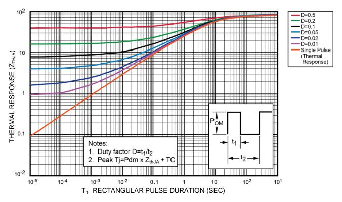
FIGURE 2 - Normalized Transient Thermal Impedance
