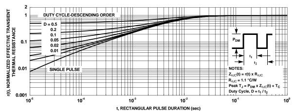
Figure 13. Transient Thermal Response Curve
