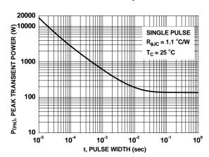
Figure 12. Single Pulse Maximum Power Dissipation
