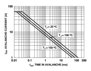
Figure 9. Unclamped Inductive Switching Capability
