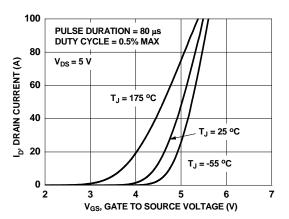
Figure 5. Transfer Characteristics
