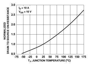
Figure 3. Normalized On-Resistance vs Junction Temperature
