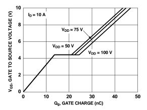
Figure 7. Gate Charge Characteristics
