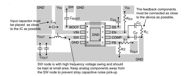
Figure 9. PCB Layout Guide
