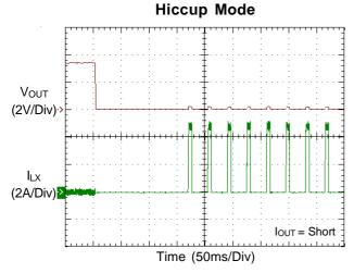
Figure 5. Hiccup Mode Under Voltage Protection
