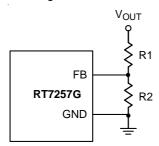
Figure 1. Output Voltage Setting
