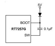
Figure 2. External Bootstrap Diode
