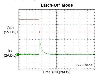
Figure 6. Latch-Off Mode Under Voltage Protection
