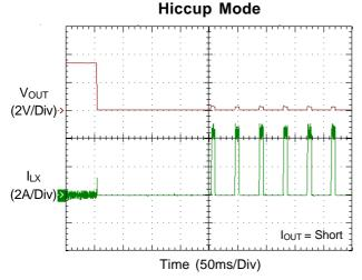
Figure 5. Hiccup Mode Under Voltage Protection
