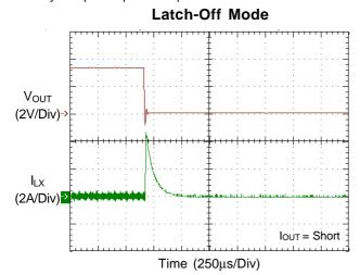
Figure 6. Latch-Off Mode Under Voltage Protection
