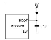
Figure 2. External Bootstrap Diode
