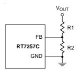
Figure 1. Output Voltage Setting
