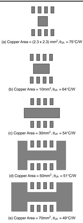
Figure 7. Thermal Resistance vs. Copper Area Layout Design
