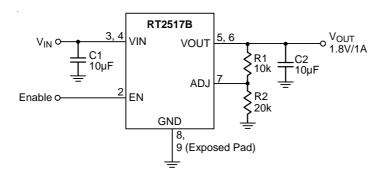
Figure 1. 1.8V Output Voltage Operation Circuit
