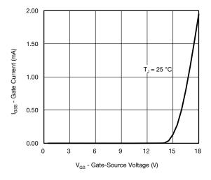
Gate Current vs. Gate-Source Voltage
