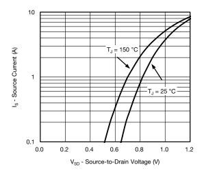
Source-Drain Diode Forward Voltage
