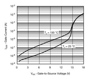
Gate Current vs. Gate-Source Voltage
