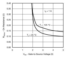
On-Resistance vs. Gate-to-Source Voltage
